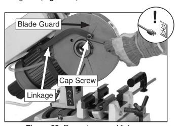
Figure 22. Removing guard linkage.
